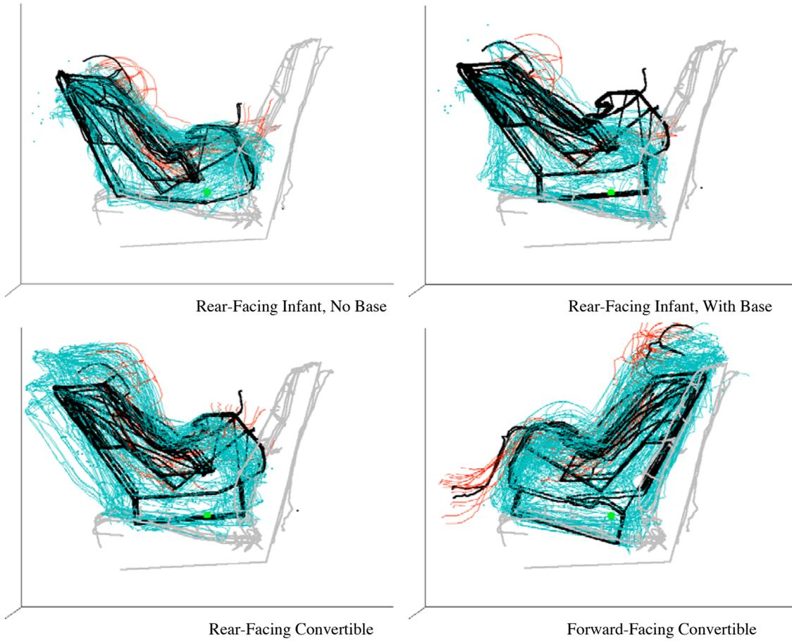
Figure 15. Overlay of convertible surrogate geometry (thick lines) with data from commercial child restraints (thin lines) in a vehicle seat.
