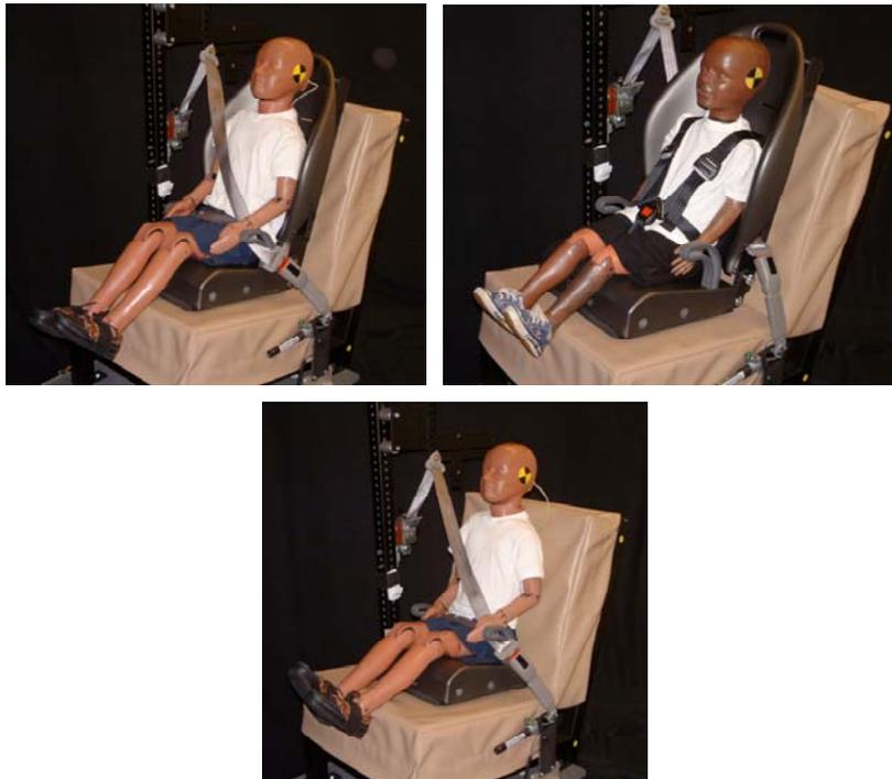
Figure 13. Final booster surrogate, from top to bottom, as a high-back booster, forward-facing-only restraint, and backless booster.
