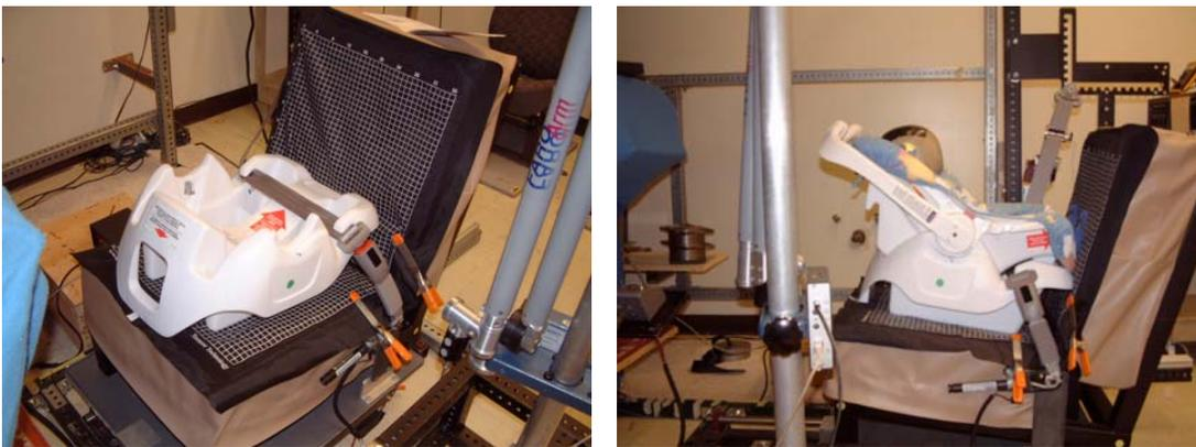
Figure 6. Xsensor pressure distribution measurement mats installed under a child restraint and on seatback.
