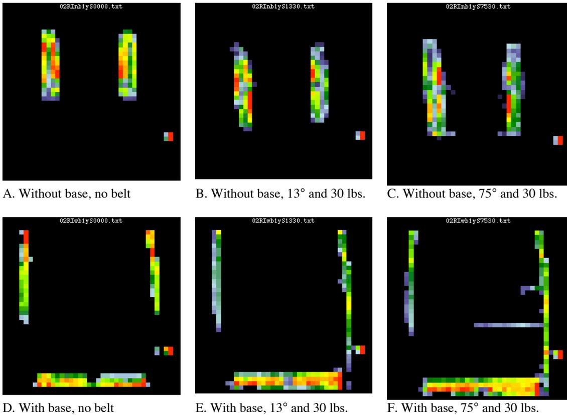
Figure 7. Example of seat surface pressure distribution for a rear-facing infant restraint in a range of belt conditions on the standard vehicle seat. Rear of vehicle seat is at bottom of images. Dot on right margin marks the fore-aft H-point location. Areas of higher pressure are shown in red and yellow; blue indicates lower pressure.
