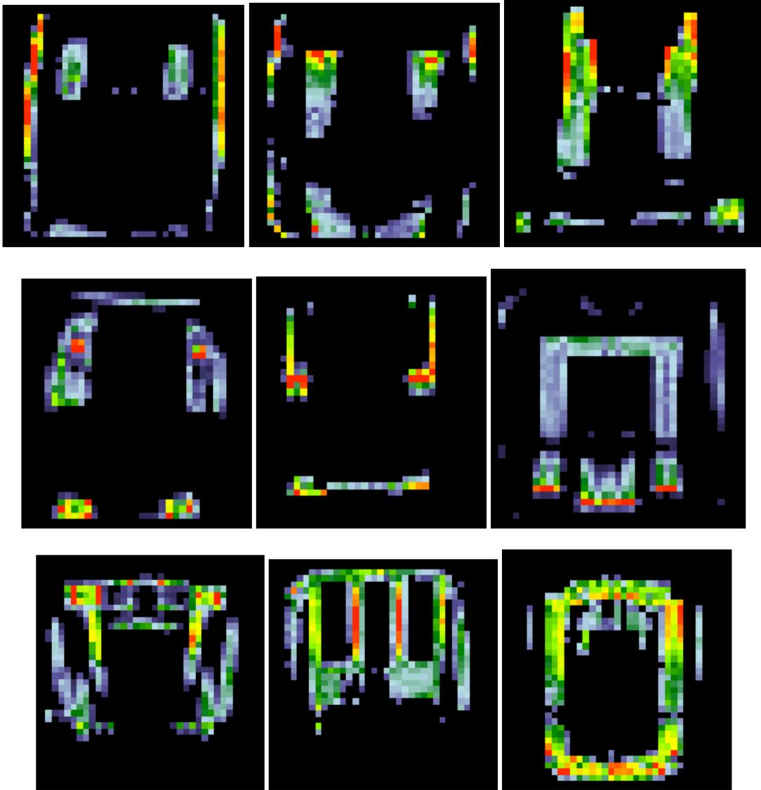
Figure 8. Pressure distributions on the seat cushion surface from selected restraints in three categories: rear-facing infant restraints (top), forward-facing convertibles (middle), and forward-facing harness and booster restraints (bottom). Red indicates areas of highest pressure, yellow and green are medium pressure values, and blue indicates low pressure. Data are from the 13-degree, 15-lb belt condition in vehicle seat number one.
