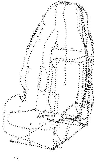
Figure 2. Data point cloud for one child restraint.
