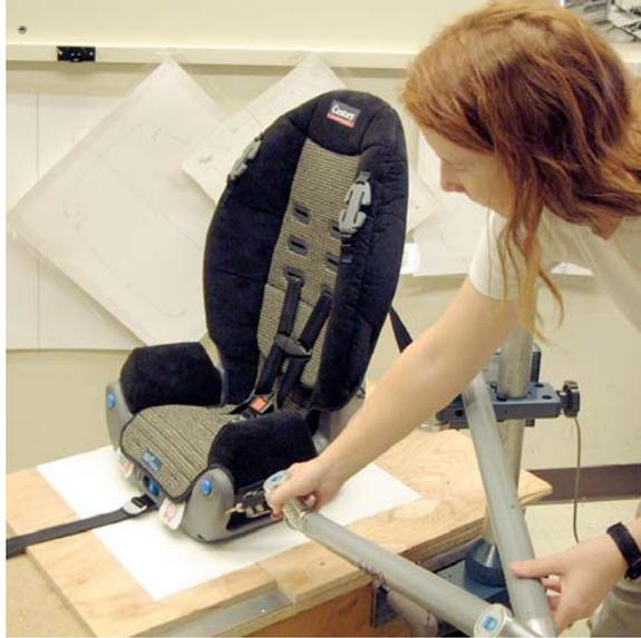
Figure 1. Digitizing child restraint geometry.
