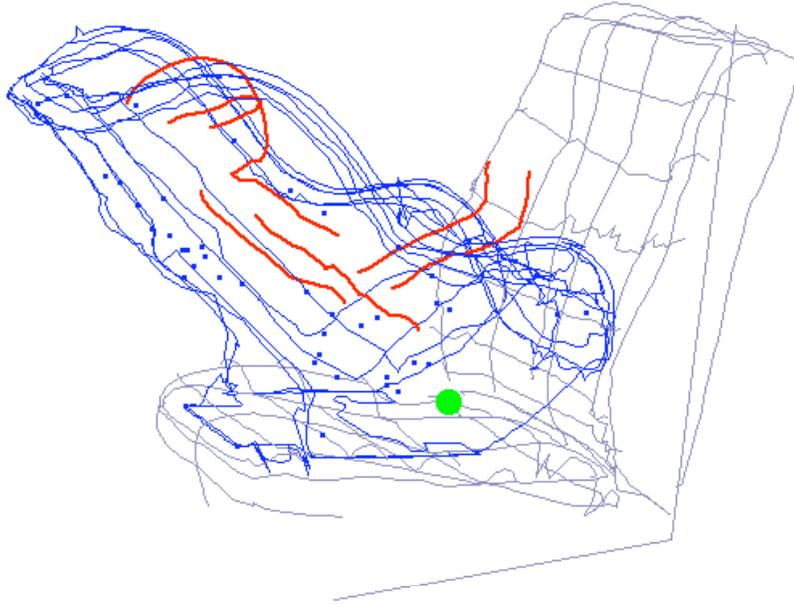
Figure 9. Geometric data from one in-seat trial obtained by combining in-seat measurements with previously measured restraint geometry aligned to reference points. Contour streams on ATD and seat surface contours are also shown. Large dot is seat H-point.
