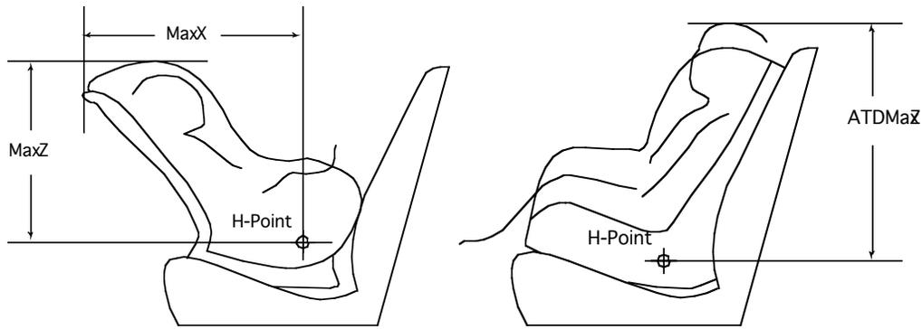
Figure 17. Schematic of dependent measures representing in-seat child restraint position.
