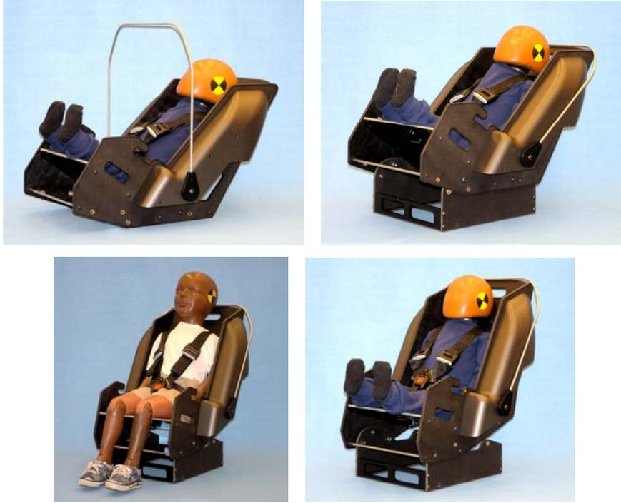
Figure 12. Final convertible surrogate prototype, from top to bottom, as a rear-facing infant seat without base, rear-facing infant/convertible with base, and forward-facing convertible with 3YO and 12-month ATDs.
