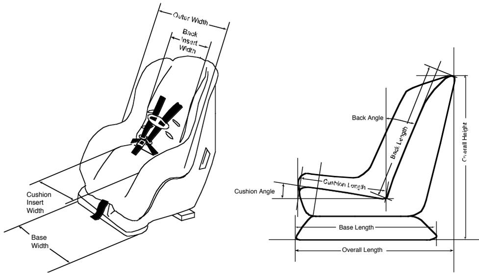
Figure 10. Definitions of child restraint dimensions in Table 6.
