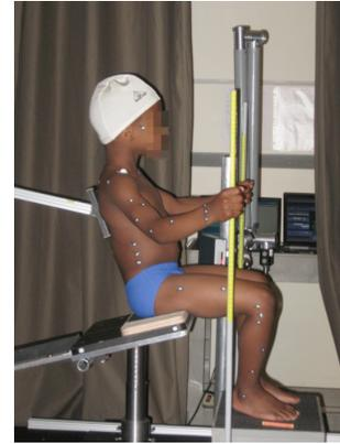
Figure 1. Child in the VITUS XXL whole-body laser scanner, showing fixtures used to support seated postures.
