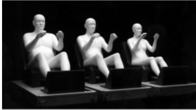
Figure 14. Large-male, midsize-male, and small-female standard reference shells developed for crash dummy anthropometry.
