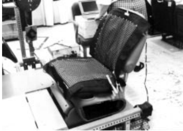
Figure 6. Pressure mapping system installed in test seat.
