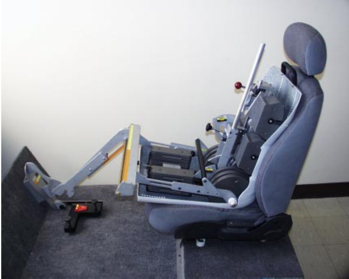
Figure 2. ASPECT manikin prototype (APM-4), shown with supplemental thigh and leg components.
