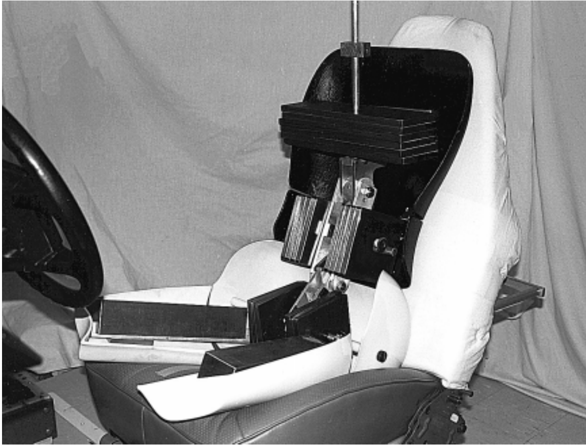
Figure 12. APM2 prototype (October 1997) showing leg splay features.
