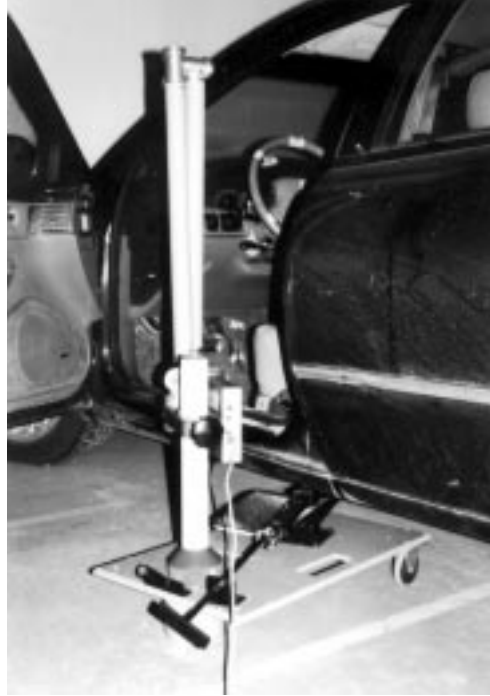
Figure 2. FARO arm digitizer hardware.
