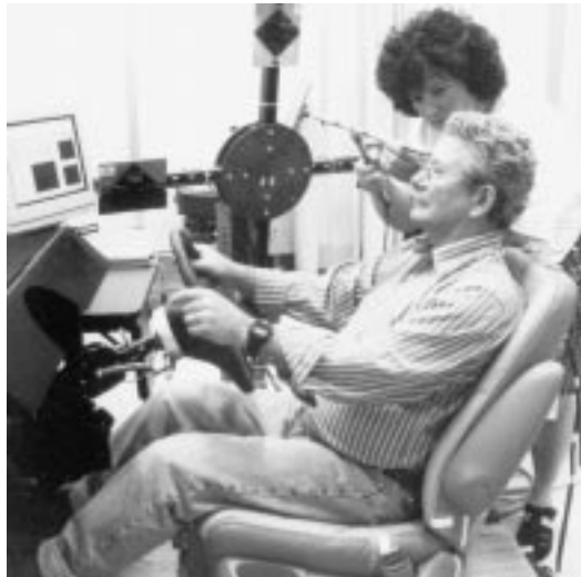
Figure 6. Digitizing a subject's body landmarks using a sonic digitizer
