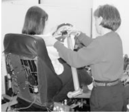
Figure 5. Digitizing a subject's body landmarks using a FARO arm.
