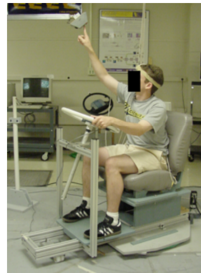
Figure 2. Participant seated in the rotating truck seat reaching towards the push-button target.
