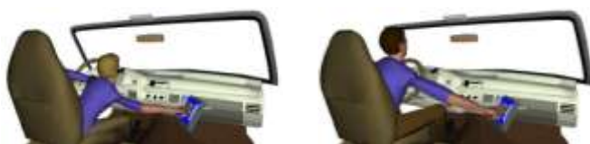
Figure 2. Virtual Driver with 5% female and 95% male drivers.
