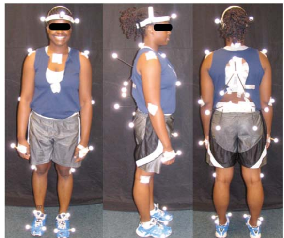
Figure 2: Retro-reflective marker set used to capture whole-body postures.
