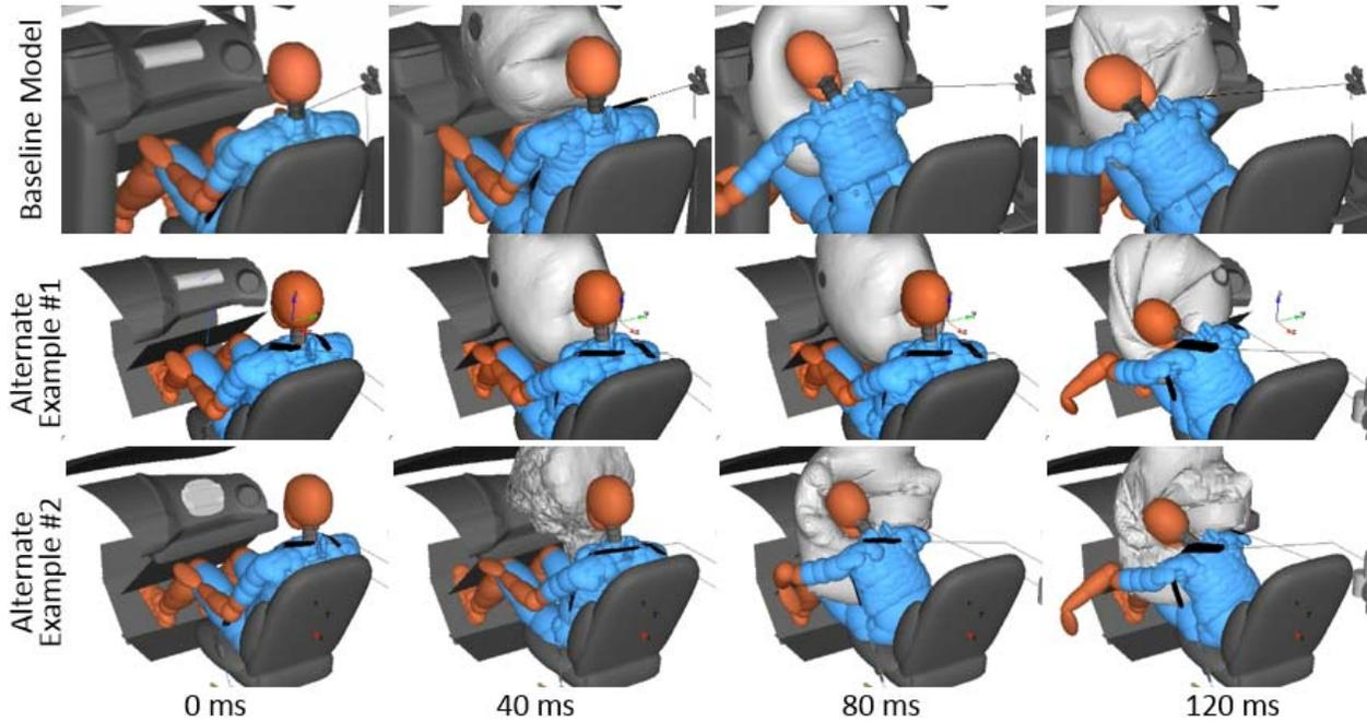
Fig. 7. THOR kinematics with the baseline restraint and two alternate PAB and prototype suspender 4-point belt designs.
