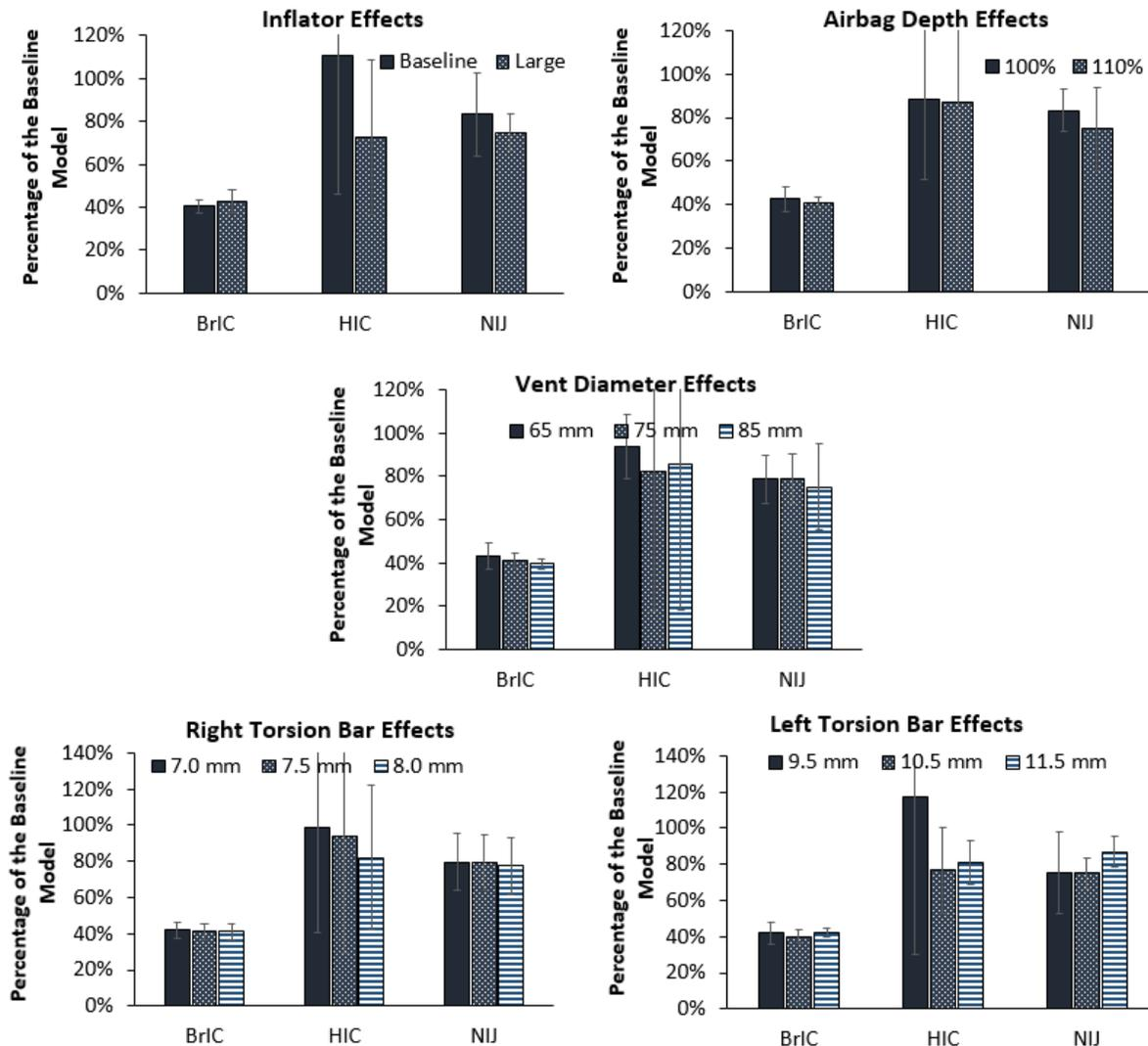
Fig. 6. Airbag and seatbelt effects on ATD injury measures in passenger far-side impacts.
