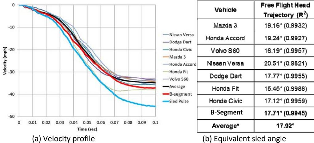
Fig. 2. Impact kinematics for eight vehicles in NHTSA oblique crash tests.
