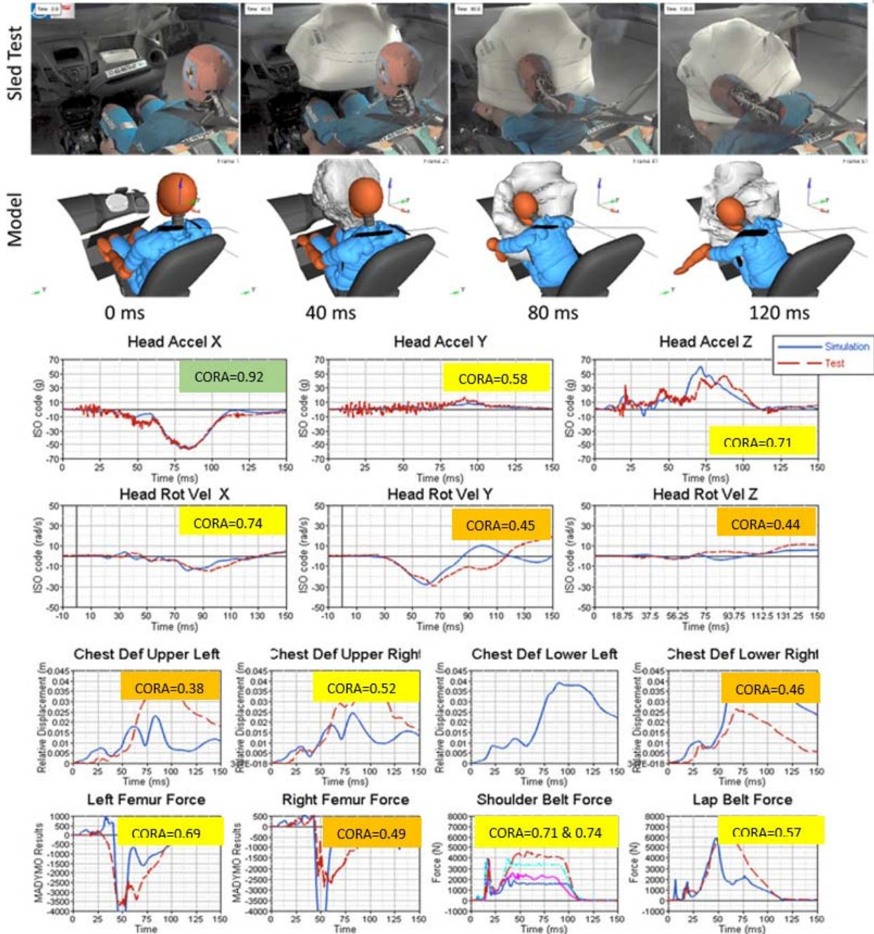
Fig. 5. Model-predicted occupant kinematics and injury measures compared with test using suspender 4-point belt.
