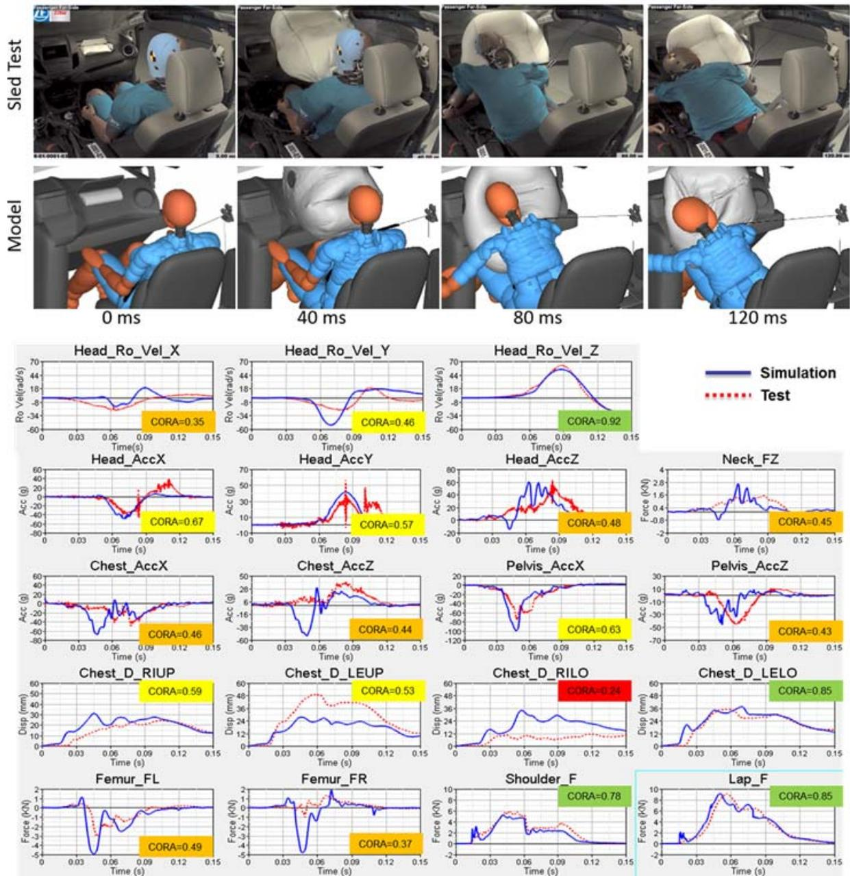
Fig. 4. Model-predicted occupant kinematics and injury measures compared with baseline test.
