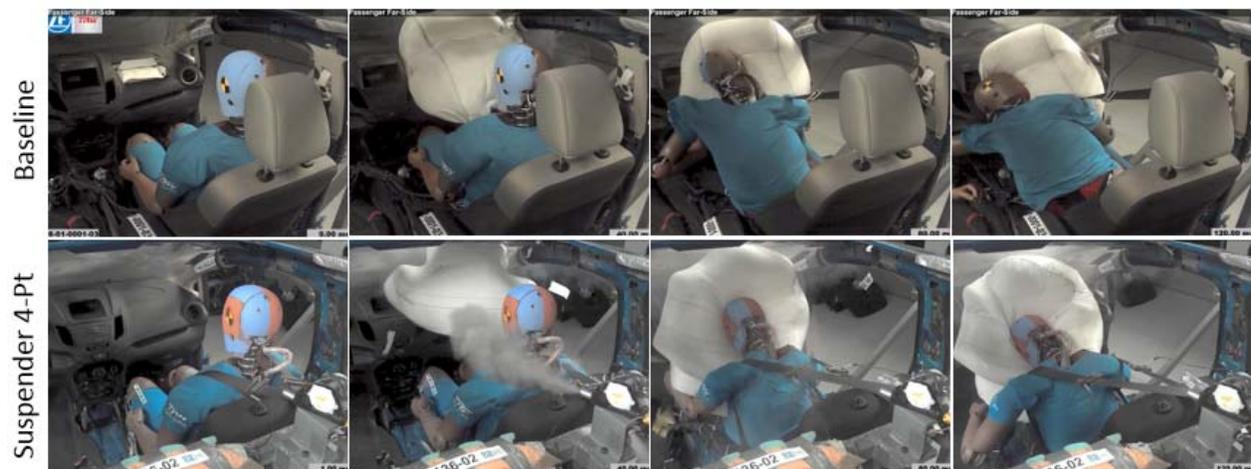
Fig. 8. Occupant kinematics in baseline and final sled tests
