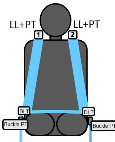
Fig. 1. Illustration of a suspender 4-point belt.
