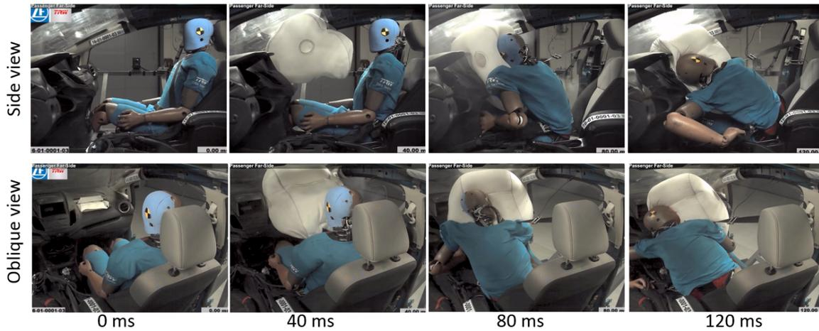
Fig. 3. Occupant kinematics in the passenger far-side baseline sled test.
