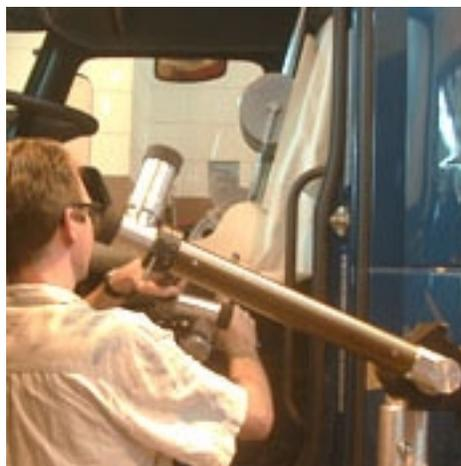
Figure 1. H-point measurement in a truck cab using the FARO Arm.
