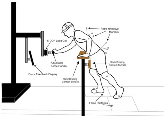
**Figure 1:** Laboratory configuration with visual force feedback display, 6-DOF load cells at task handle and bracing obstructions, and reconfigurable force platforms for measuring forces and moments at the hand and feet respectively.
