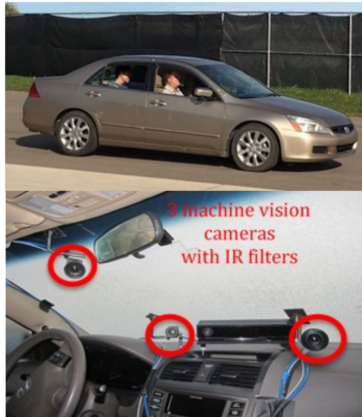
Fig. 3.1 Test vehicle exterior (left) and interior camera placement (right)
