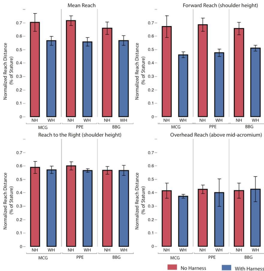
Figure 3. Mean, forward, right, and overhead reach distances ( $\pm$  standard deviation)
