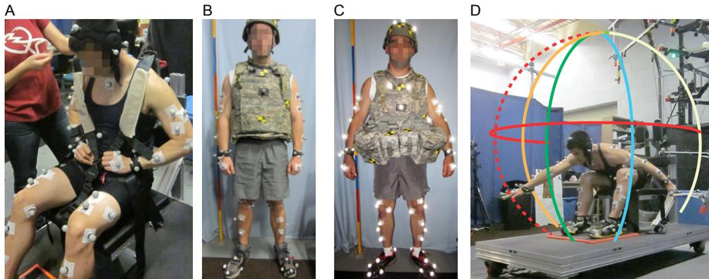
Figure 1. Participant donning 5-point harness in minimally clad garment (MCG: A). Participant wearing PPE (B) and BBG (C). The “virtual” traces of maximal reach motions (D).
