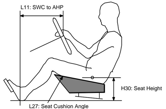
Figure 10. Illustration of inputs to ATD Positioning Model.
