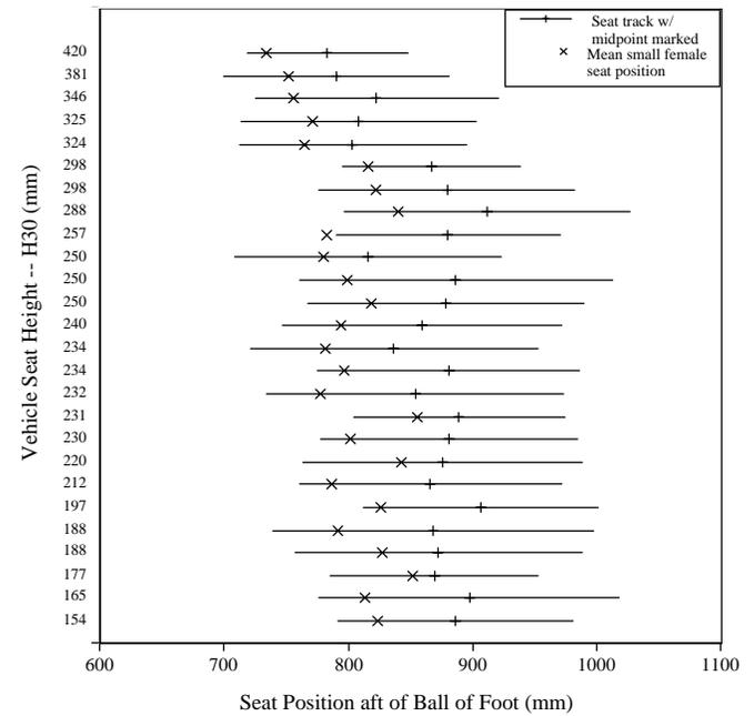
Figure 3. Mean small female seat position relative to the seat track in 26 vehicles. Vehicles are rank-ordered by seat height (H30) on the vertical axis.
