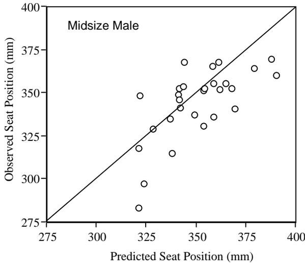
Figure 11b. Seat positions (H-points locations) aft of steering-wheel center predicted by the ATDPM, compared with observed mean seat positions for midsize-male drivers in 30 vehicles.
