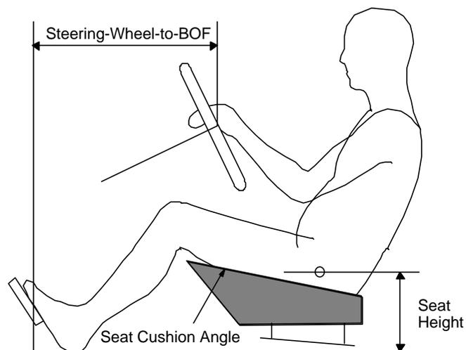
Figure 9. Illustration of vehicle and seat factors used as input to the Seating Accommodation Model.
