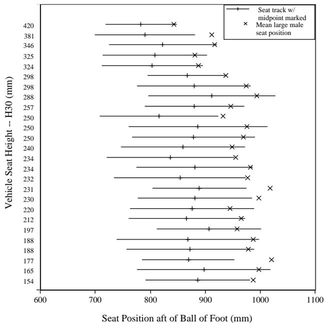
Figure 4. Mean large male seat position relative to the seat track in 26 vehicles. Vehicles are rank-ordered by seat height (H30) on the vertical axis.
