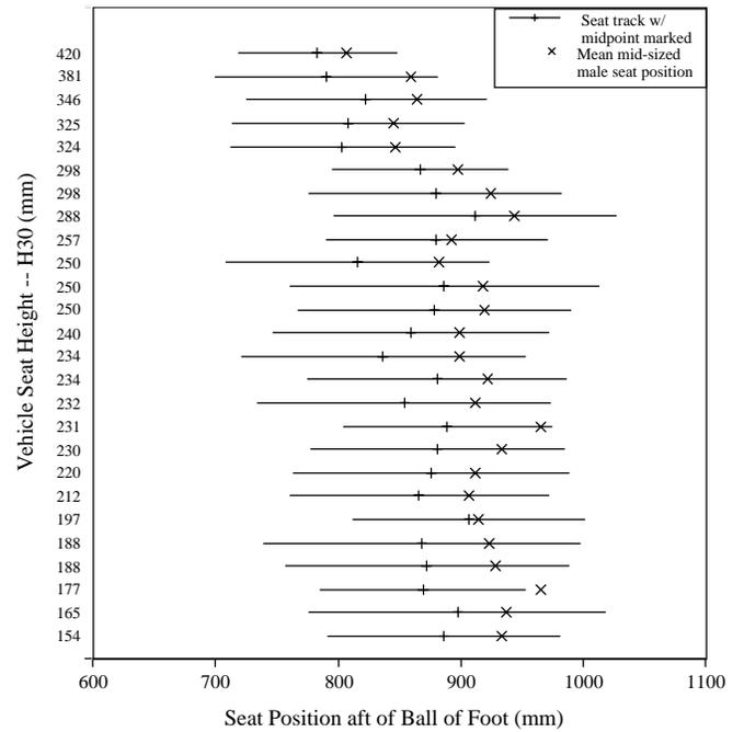
Figure 2. Mean midsize male seat position relative to the seat track in 26 vehicles. Vehicles are rank-ordered by seat height (H30) on the vertical axis.
