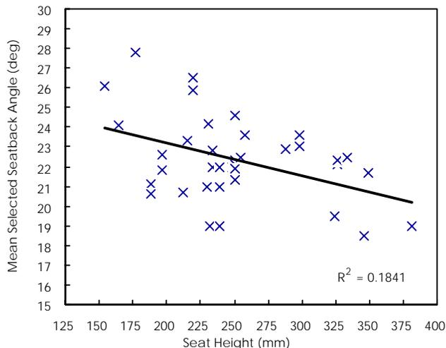
Figure 6. Relationship between seat height and mean selected seatback angle for 37 vehicles.
