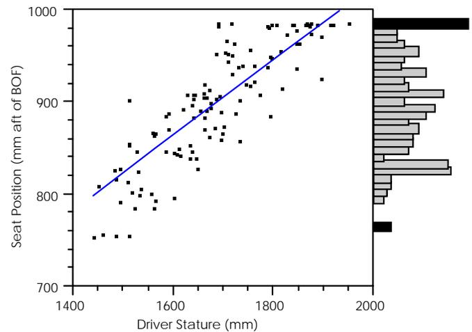
Figure 1. Relationship between stature and seat position for 120 drivers in one vehicle. Dark bars on seat position histogram indicate censored observations at the ends of the seat track travel. Linear regression, excluding the censored observations, gives  $R^2 = 0.67$ .
