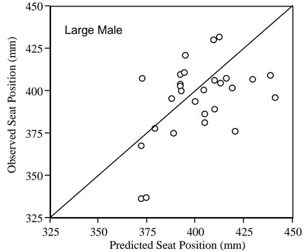
Figure 11c. Seat positions (H-points locations) aft of steering-wheel center predicted by the ATDPM, compared with observed mean seat positions for large-male drivers in 30 vehicles.
