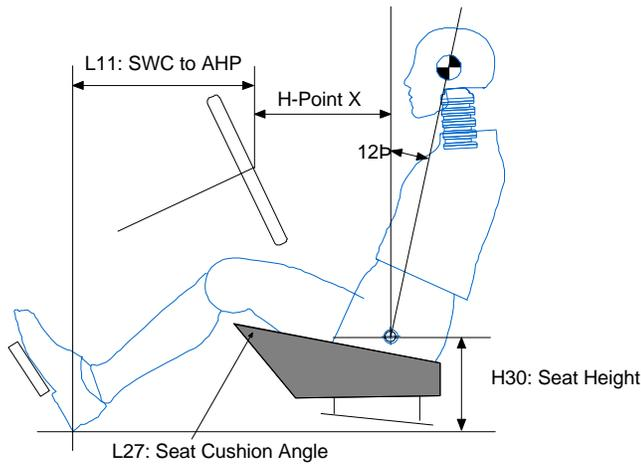
Figure 12. Schematic showing application of ATDPM.
