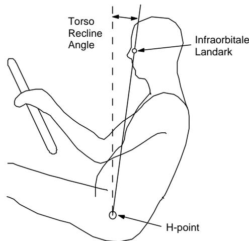
Figure 7. H-point-to-eye vector used to measure overall torso recline angle.
