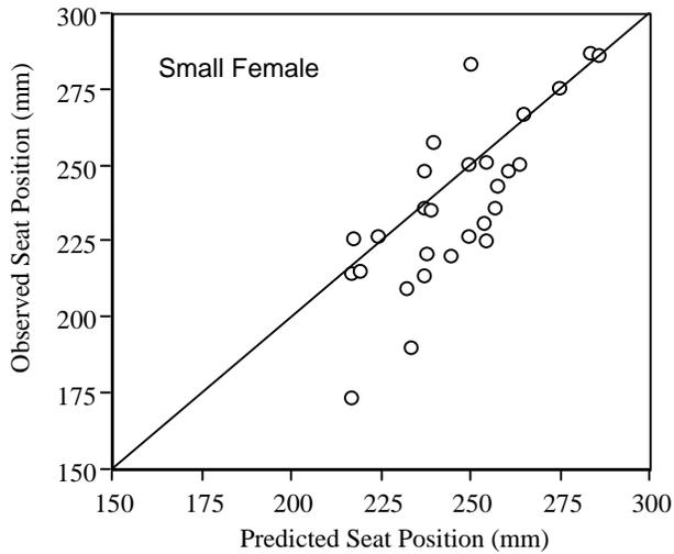
Figure 11a. Seat positions (H-points locations) aft of steering-wheel center predicted by the ATDPM, compared with observed mean seat positions for small-female drivers in 30 vehicles.
