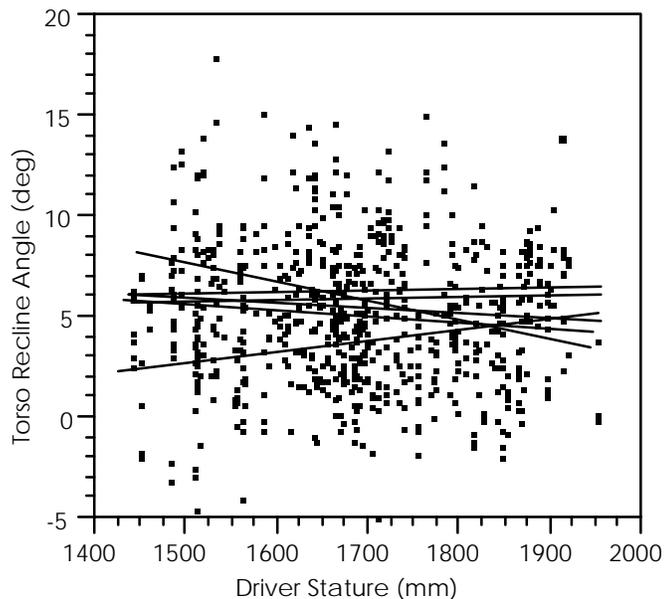
Figure 8. Relationship between stature and torso recline for six vehicles, 113 to 120 subjects per vehicle. Lines are linear fits to the data from each vehicle.
