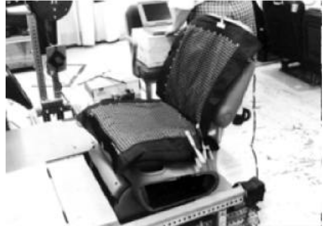
Figure 6. Pressure mapping system installed in test seat.
