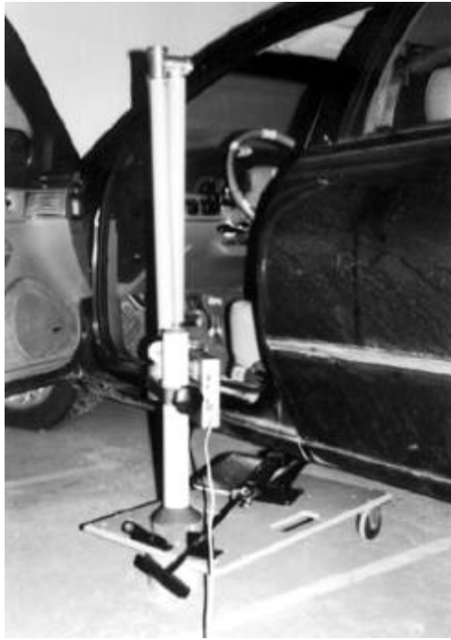
Figure 2. FARO arm digitizer hardware.
