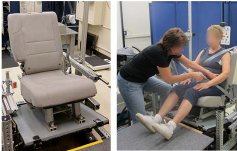
Fig. 1. Reconfigurable rear seat mockup and recording a participant's ASIS landmark location using a FARO Arm coordinate digitiser.
