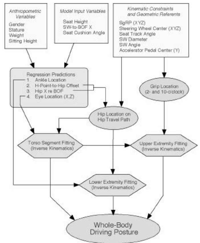
Figure 3. Schematic of Cascade Prediction Model (CPM).
