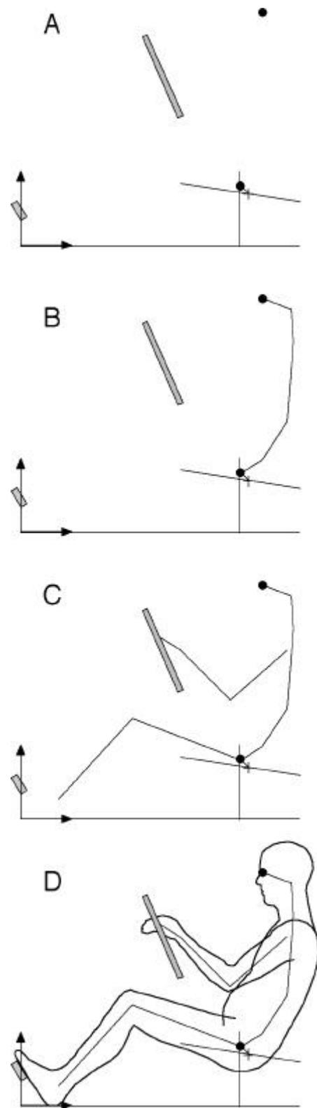
Figure 4. Step-by-step illustration of Cascade Prediction Model approach to predicting driver posture. A: Predict hip and eye locations; B: Fit torso segments by inverse kinematics using data-based motion distribution; C: Fit limb segments by inverse kinematics using splay data; D: Fit full 3-D model to kinematic linkage.
