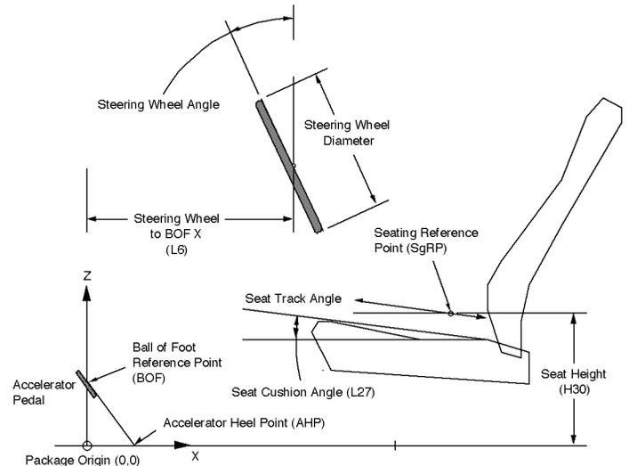
Figure 1. Vehicle package geometry. Expressions in parentheses are Society of Automotive Engineers nomenclature from SAE J1100 (3).
