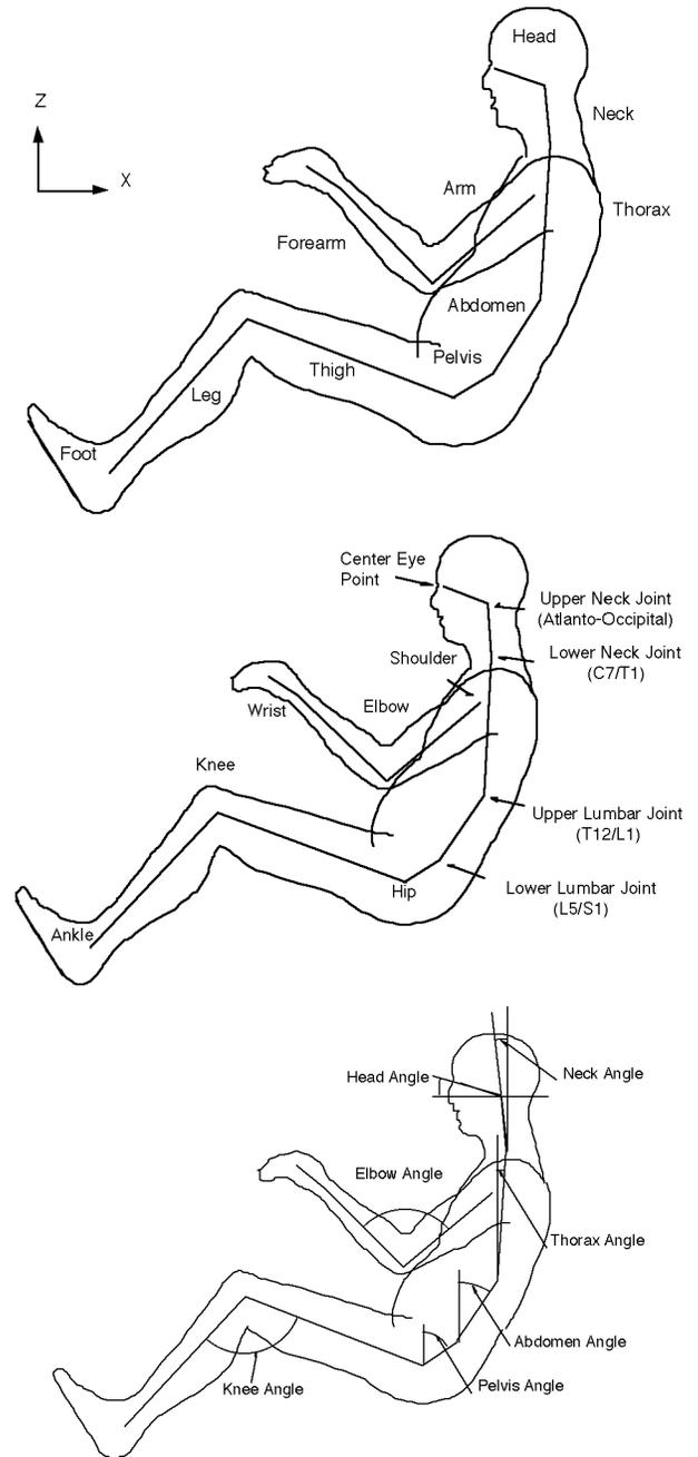
Figure 2. Definitions of kinematic linkage and posture measures (12). Angles referenced to horizontal or vertical are XZ (sagittal) plane angles. Angles between segments (elbow angle, knee angle, and ankle angle) are measured in the plane formed by the segments (included angles). Note: Neck angle is negative as shown. All other angles are positive as shown.
