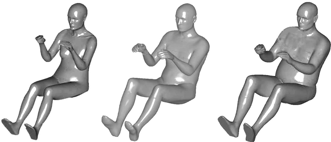
Figure 10. Small female, midsize male, and large male body surface contours for representing humans in CAD environments
