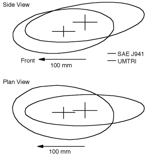
Figure 4. Comparison of SAE J941 and new UMTRI 95<sup>th</sup>-percentile eyellipses for a typical vehicle geometry and 50-percent-male U.S. driving population.
