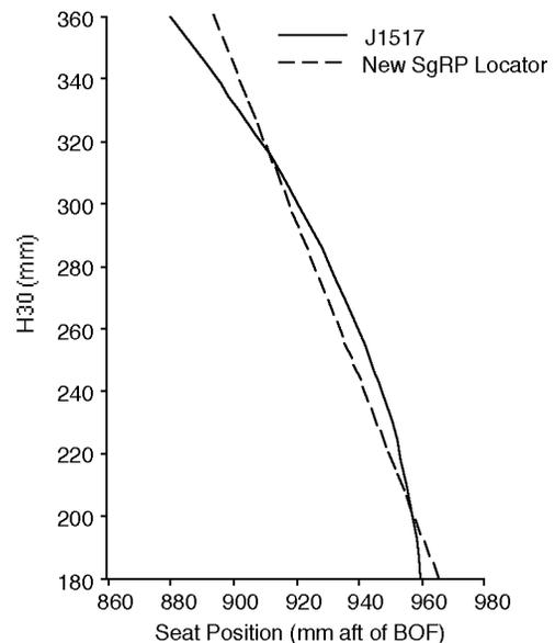
Figure 8. Comparison of proposed SgRP locator function with currently used SAE J1517 95<sup>th</sup>-percentile driver-selected seat position curve.
