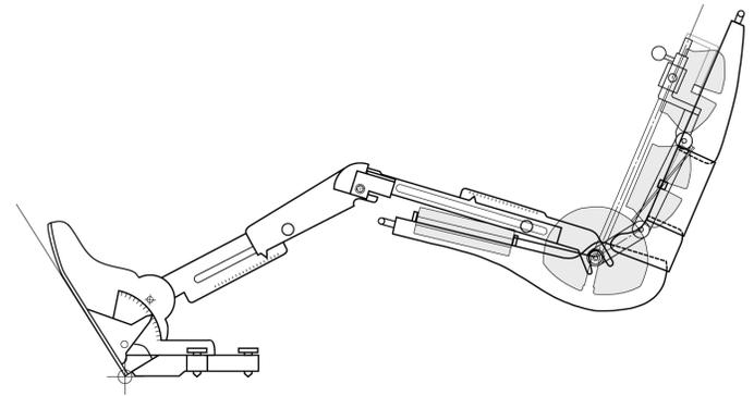
Figure 5. New ASPECT manikin, shown with supplemental thigh, leg, and shoe components (9).
