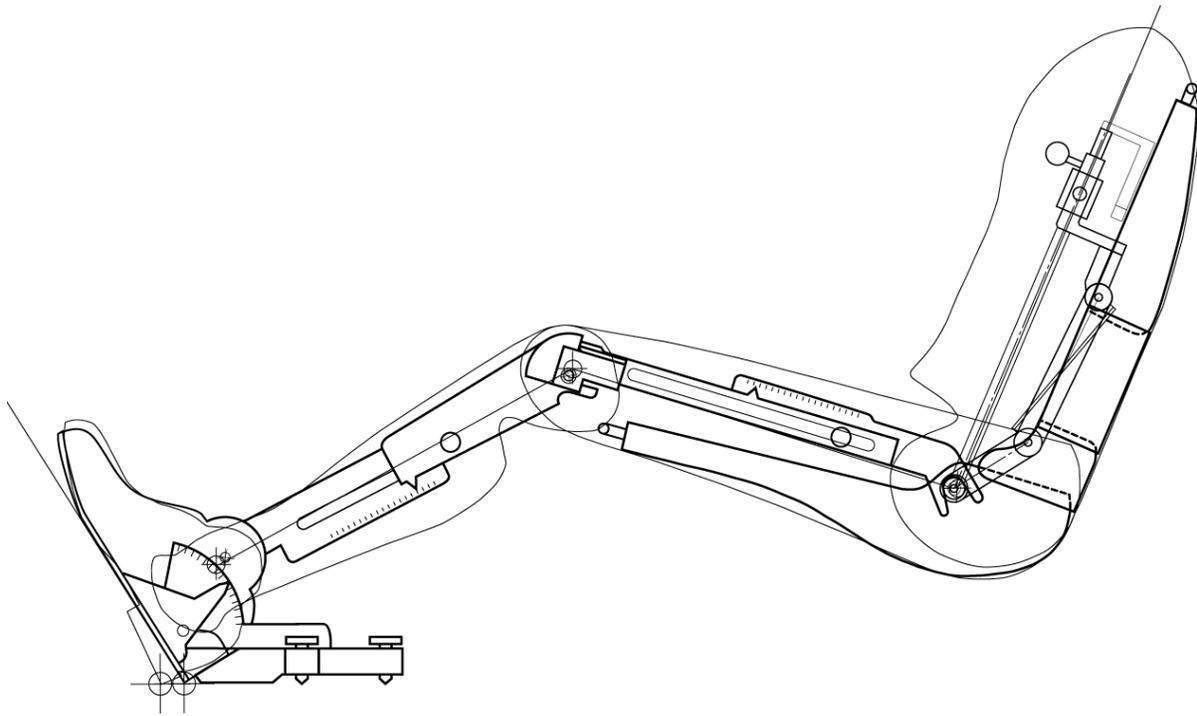
Figure 9. Comparison of current (light lines) and new (ASPECT manikin) packaging practices for a 220-mm seat height.
