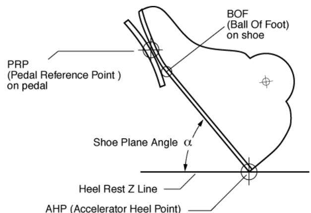
Figure 7. Manikin shoe oriented according to the calculated shoe plane angle ( $\alpha$ ) on a pedal oriented according to the current SAE J1516 pedal plane angle function.
