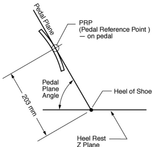
Figure 6. Proposed procedure for locating a pedal reference point (PRP) on the accelerator pedal.
