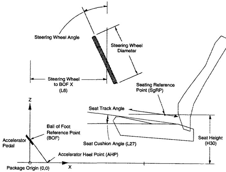
Figure 1. Vehicle package geometry. Expressions in parentheses are Society of Automotive Engineers nomenclature from SAE J1100 (SAE, 1997).
