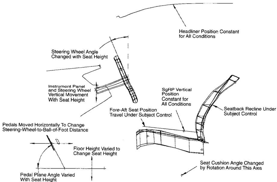
Figure 2. Schematic of vehicle mockup showing adjustment axes.
