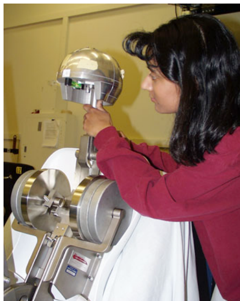
Figure 2. Head Restraint Measurement Device mounted on the SAE J826 H-point machine.
