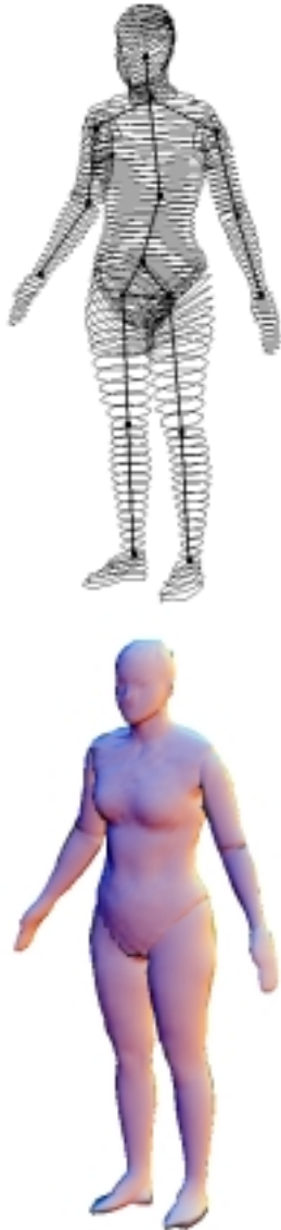
Figure 3. Slice planes used to create quadrangle meshes on each segment (above) and the resulting whole-body model (below).
