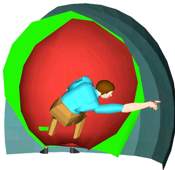
Figure 4. Expansion of reach capability obtained by rolling the pelvis (compare with Figure 3).
