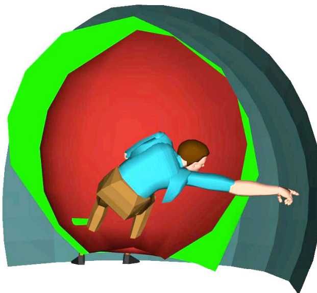
Figure 5. Expansion of reach capability obtained by rolling pelvis and releasing limits at sternoclavicular joint to better approximate the observed (outermost) reach envelope.
