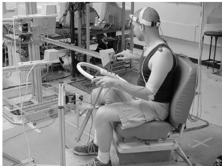
Figure 1. Laboratory setup, showing the optical and electromagnetic markers used to track motions and the computer-controlled target-positioning apparatus.
