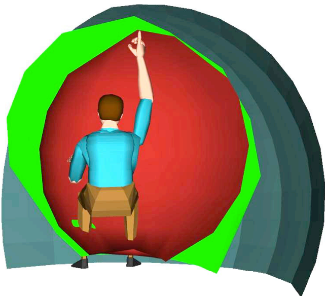
Figure 2. Illustration of posture on boundary of maximum reach envelope generated using mobility starting at the sternoclavicular joint (innermost envelope).
