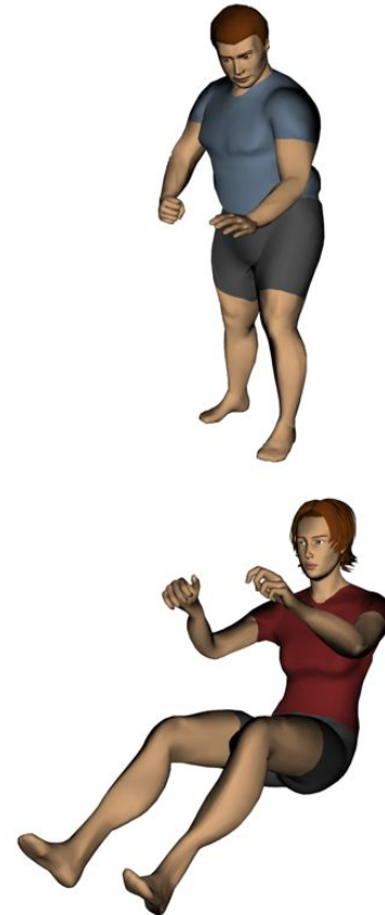
Figure 3. Male and female figures in the Jack human modeling software system generated from the statistical body shape models based on laser-scan data.
