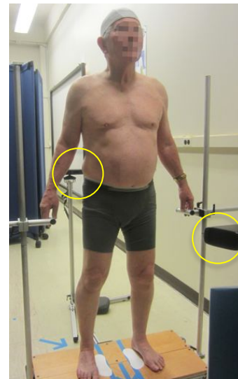
Figure 1. Hardware system with Kinect sensors to record the front and back of the subject. Circles show the sensor locations.
