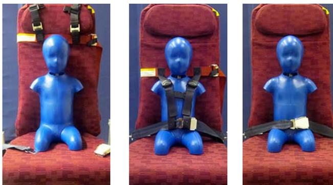
Fig. 2. Manikin in an aviation seat.
