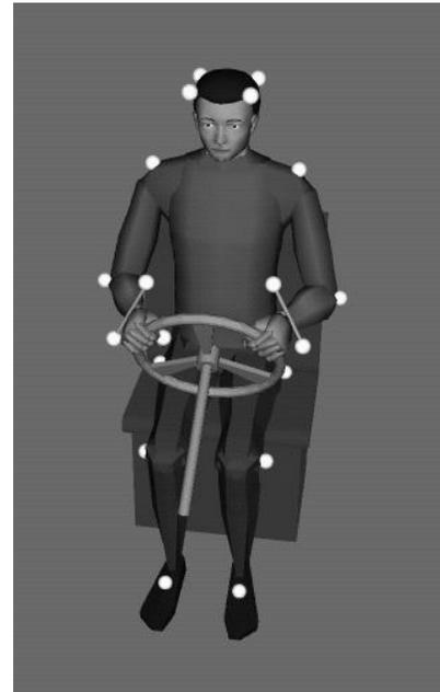
**Figure 5. Jack digital human showing reflective marker locations.**
