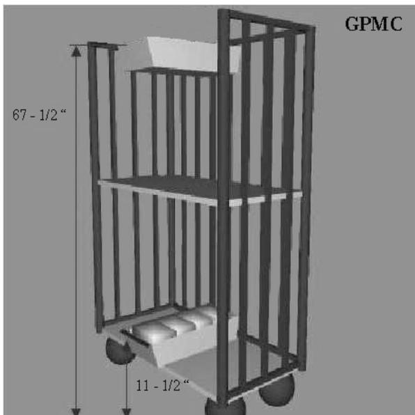
**Figure 1. Dimensions of extreme tray heights in the General Purpose Mail Cart (GPMC).**
