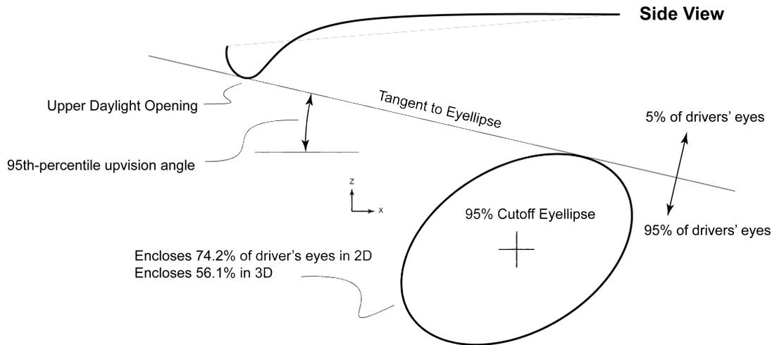
Figure 1. Illustration of side-view eyellipse with 95% cutoff characteristic.
