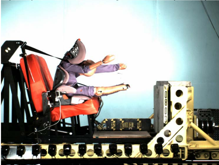
Figure 17. Peak excursion in test using TurboBooster and poor lap belt geometry.
