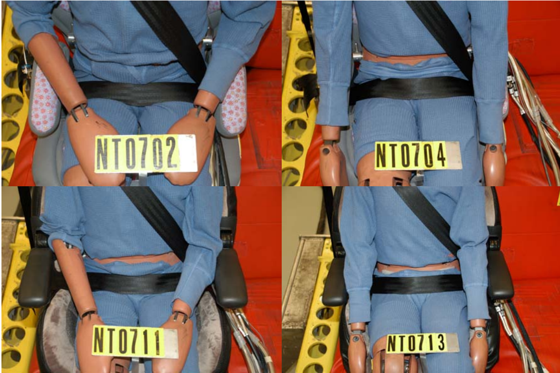
Figure 11. Initial lap belt position on TurboBooster (top row) and Generations (bottom row) using FMVSS 213 seating procedure (left) and UMTRI seating procedure (right). The front edge of the belt is trapped in the gap in test NT0702.
