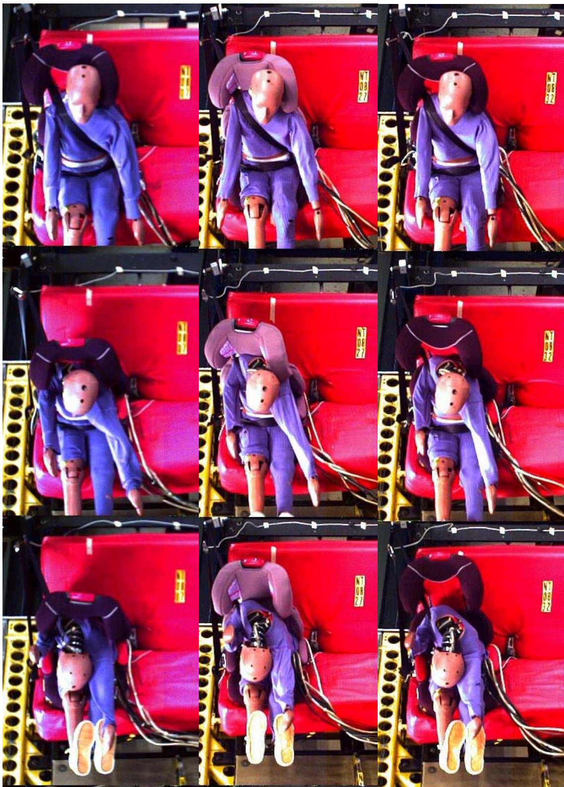
Figure 25. Kinematics of TurboBooster (left), TB with modified slot (middle), and rigid TB. Frames from top to bottom are from times 80, 100, and 120 ms.
