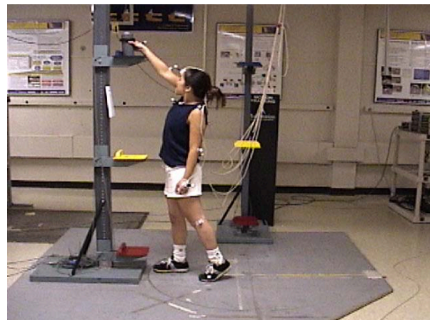
Figure 1. Participant in test facility layout, shelving tower 1 and 2, and motion capture hardware. Participant is shown at tower 1.
