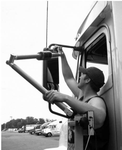
Figure 1. Digitizing a heavy truck mirror with the FARO Arm.
