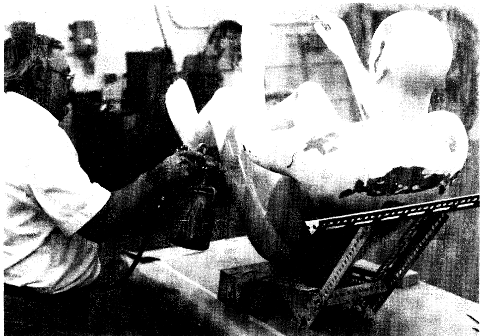
FIGURE 4-17. Finishing and painting the assembled shells.
