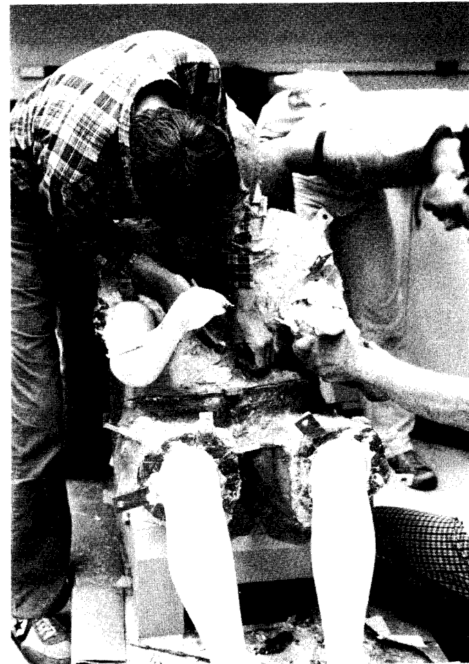
FIGURE 4-16. Removing mold parts from assembled shell.
