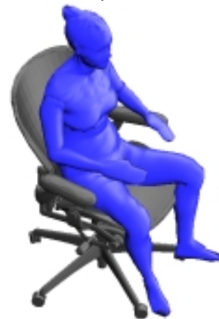
Figure 4. Whole-body model created from a standing body scan used to evaluate office chair dimensions.
