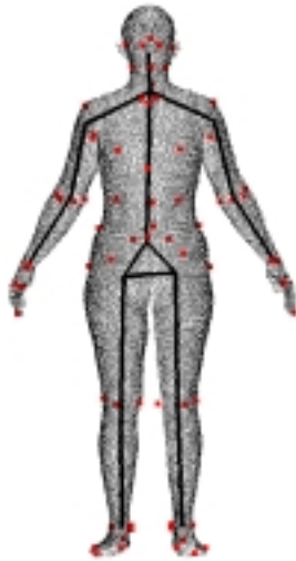
Figure 1. Point cloud from a standing scan with landmarks, calculated joint locations, and kinematic linkage (only 1/10 of sampled surface points are shown).
