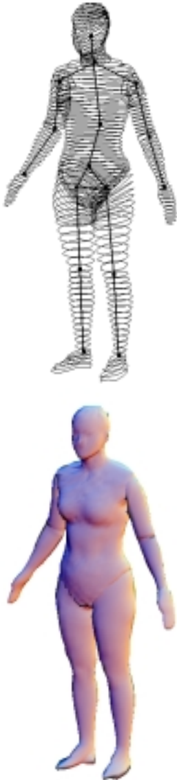
Figure 3. Slice planes used to create quadrangle meshes on each segment (above) and the resulting whole-body model (below).
