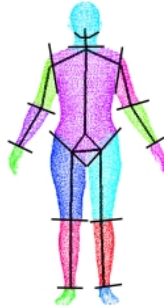
Figure 2. Scan data and skeleton with schematic illustration of segmentation planes. Actual segmentation uses multiple surfaces for some joints.
