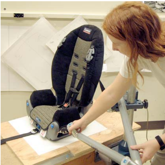
Figure 1. Digitizing child restraint geometry.
