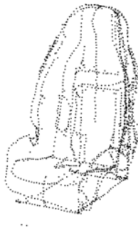
Figure 2. Data point cloud for one child restraint.
