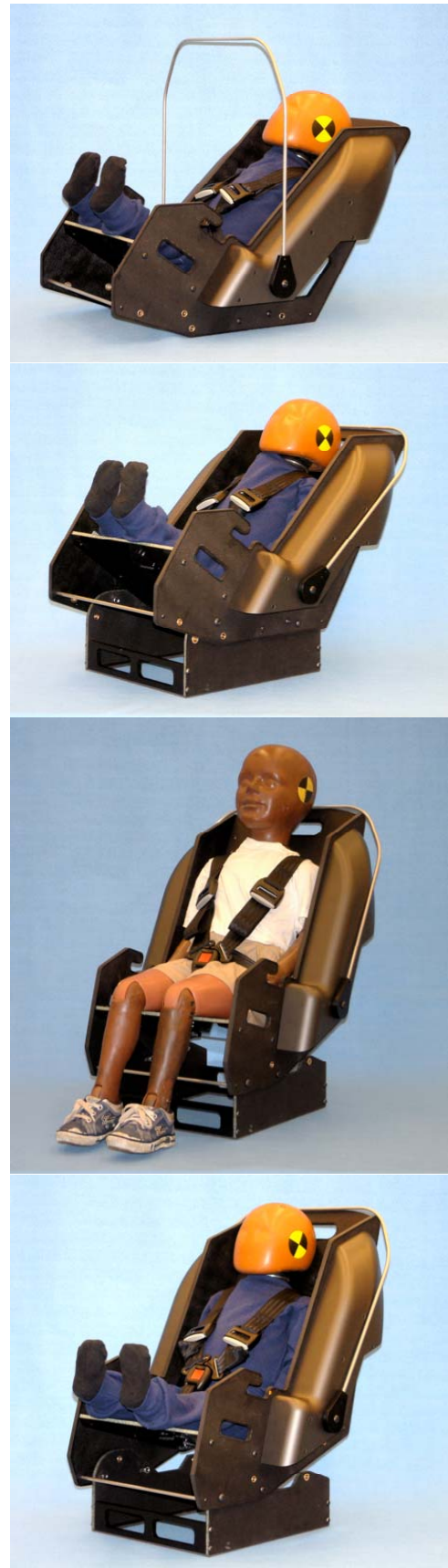
Figure 8. Final convertible surrogate prototype, from top to bottom, as rear-facing infant seat without base, rear-facing infant/convertible with base, and forward-facing convertible with 3YO and 12-month ATDs.
