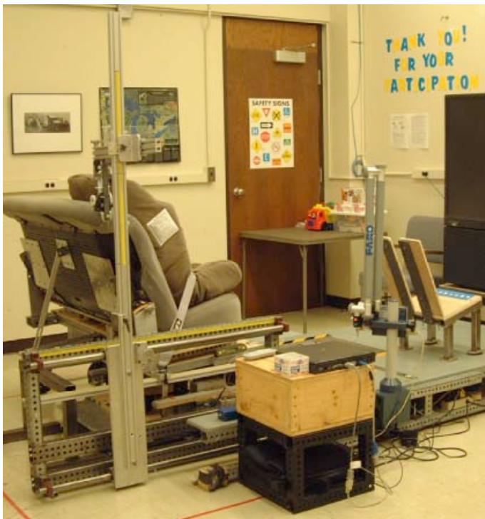
Figure 1. Reconfigurable vehicle rear-seat mockup in laboratory. The FARO Arm coordinate measurement device is visible at the right side of the picture.
