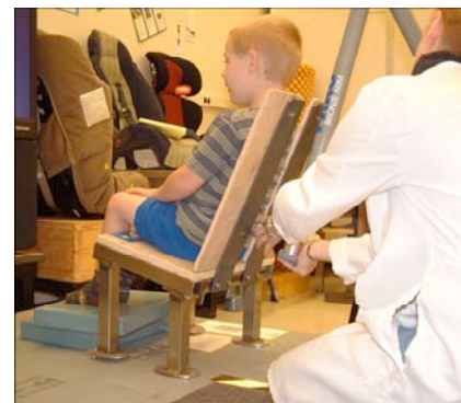
Figure 6. Participant seated in a laboratory hardseat used to obtain posterior and anterior body landmarks in same posture. A slightly larger hardseat was used with the larger participants.
