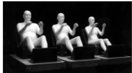
Figure 14. Large-male, midsize-male, and small-female standard reference shells developed for crash dummy anthropometry.
