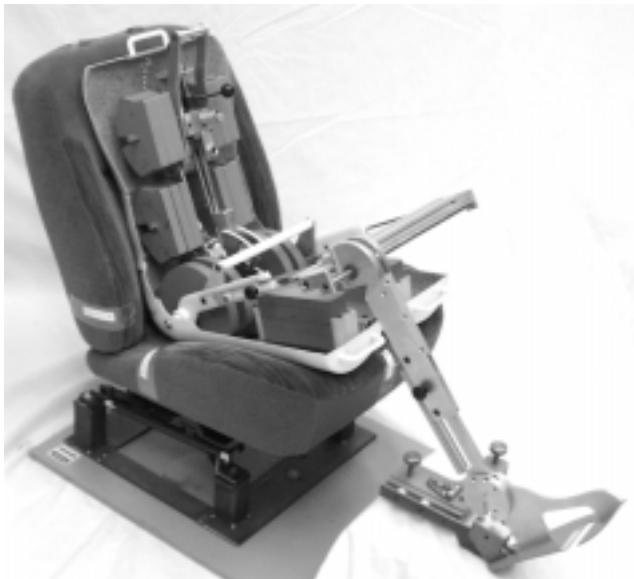
Figure 13. ASPECT manikin with thigh and leg segments installed between H-point and foot tool.
