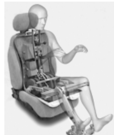
Figure 15. Midsize-male reference form and ASPECT manikin
