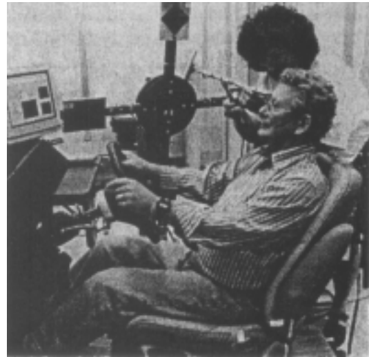
Figure 6. Digitizing a subject's body landmarks using a sonic digitizer
